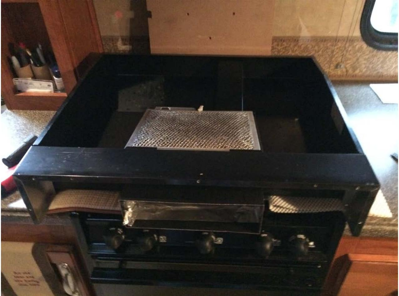
The old hood is ready for the removal of the fan box. The clip holding the light bulb in came loose and the bulb melted a hole in the old cover. At his point I disconnected the fan box wires from the switches mounted on the front of the hood. The wires to and from the switches are all connected to the black wire we cut earlier.
