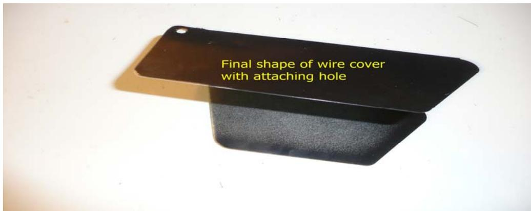
This process took a lot of time with some special tools. Those tools included: A dremel, grinder, rotary wire brush, hack saw, and file. *Of course safety glasses!* A screw in the fan kit was removed and then used to secure the wire cover.
